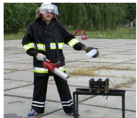
Pict.9. At first all over World – instant for 1sec: extinguishing local fires at area of 15m 2 with 2kg dust and 1,1m 2 scorched wood with single liter of clean water.
