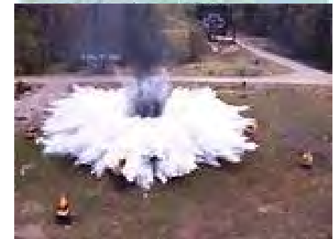
Pict.2. "TSA-500" blow flame at area up to 1000m2, but after 5-10min there can be re-inflamations
