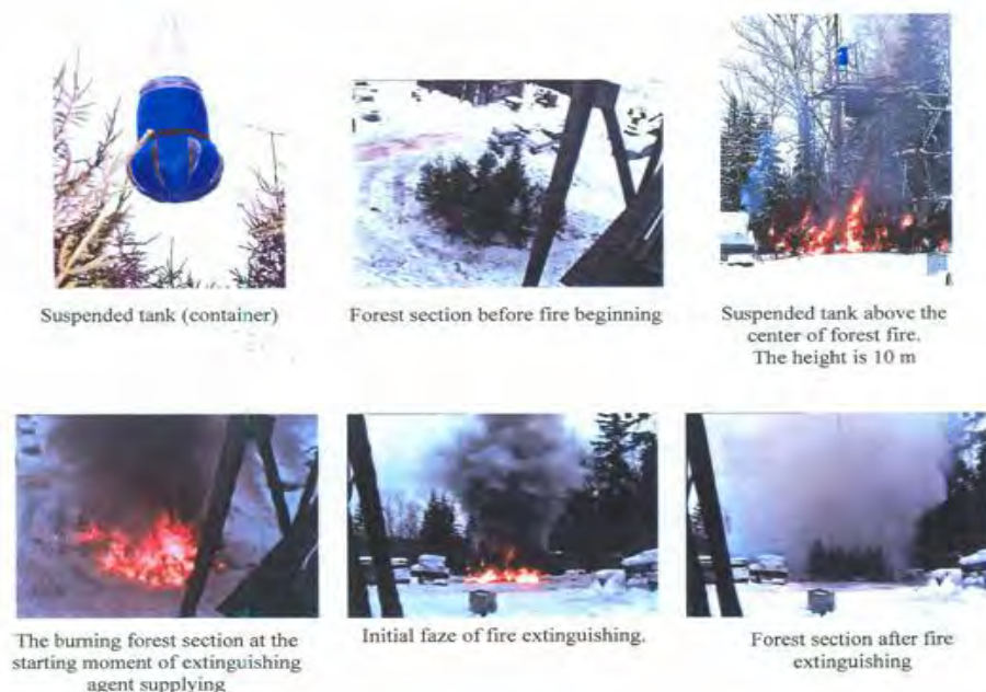
Pict. 4. Water bomb 220liters water capacity (WB-220) from 20m height ensure forest fire-fighting at 310m 2 (diameter = 20m) of pines forest of 3-5m height.
