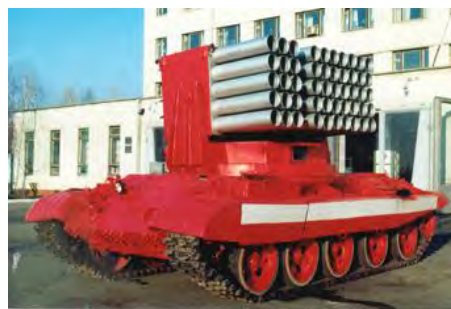
Pict. 10. Multibarrels unit on the tank-chassis for protection of military, industry, government, nuclear power stations, villages, cottages, suburbs from forest-fires.
