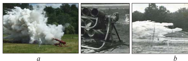
Fig. 2. a -pneumatic-pulse single-barrel module is used to arm Gazprom's emergency squads to extinguish gas wells. b -first 8-barrel module on skids, spraying with shots and volleys, in-volley of 8 barrels, spraying 120 kg of powder at a range of up to 60m with a quenching area of up to 350 m 2
