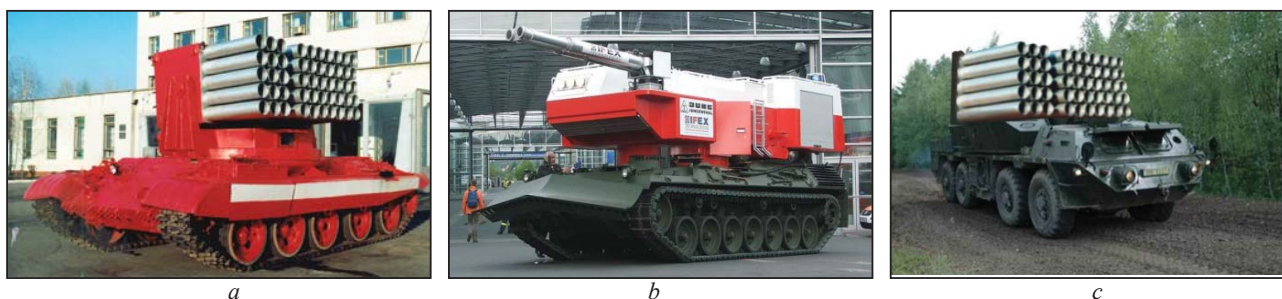
Fig. 6. A – caterpillar, armored, fire engine “Impulse-3M” with a 50-barrel tower module on the chassis of the Soviet tank “T-62”, $ 120.000; b – two-barrel “gun” IFEX-30x on the chassis of the German tank “Leopard-1”, 1.400.000 $; multi-barrel module on the chassis of the Czech wheeled tank “Dana”, 950.000 $
