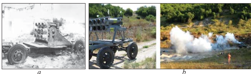
Fig. 3. A -recoil spraying 9-barrel module on a biaxial gun carriage, spraying up to 180 kg of OP for a range of up to 90 m with an extinguishing area of up to 600 m 2 , a 10-barrel deck module, spraying 12,5 kg of biosorbent with a volley from the barbs, a range of 53–55 m, area of 450 sq. m
