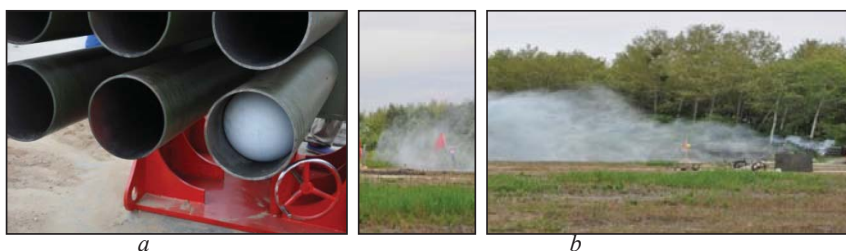
Fig. 4. A – a one-time container with a capacity of 20 liters in the barrel channel of the multi-barrel module, b – spraying 60 liters of water at a range of up to 70 m with a volley from the canals
