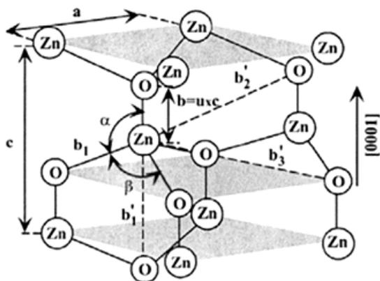
Fig. 2. Schematic diagram of Wurtzite structure of ZnO [1]
