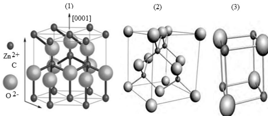
Fig. 1. Different crystalline structures of zinc oxide: (1) – wurtzite, (2) – zinc mixture, (3) – rock salt
