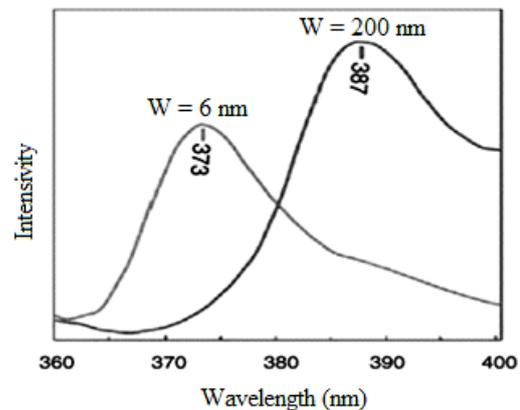
Fig. 3. Photoluminescent spectra of ZnO nanobands of wide 6 nm and 200 nm [18]
